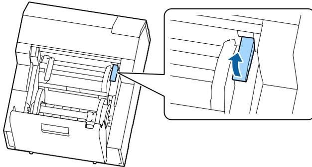
**9** Pull the paper out from the paper feed slot.
