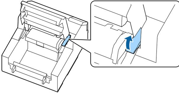
**5** Open the paper guide unit.
