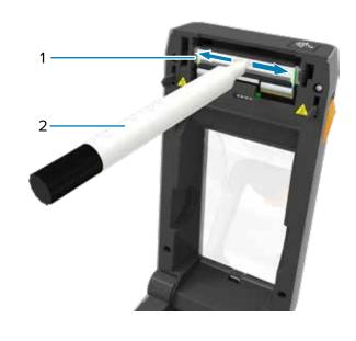
Clean printhead (1) with a cleaning pen (2). Clean from the middle to the outside. The cleaning pen is only for cleaning a printhead.
