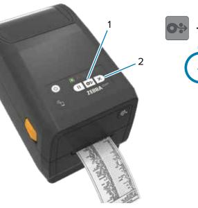
Press and hold the Feed (1) and Cancel (2) buttons for two seconds to print
