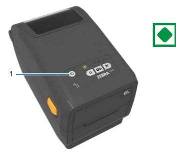
When the the printer is ready, the printer status light (1) will turn green.
