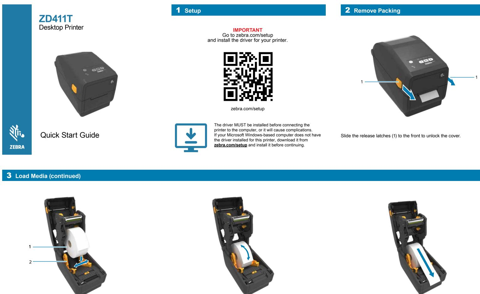
Spread the roll holders (2) open and place the roll (1) into the printer.
