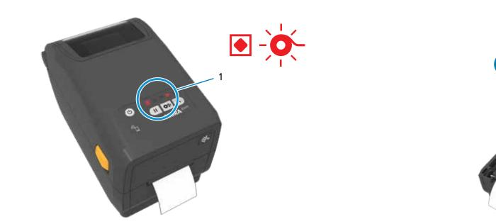
When the ribbon runs out, the printer status and a flashing media status lights (1) will turn red.
