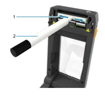
Clean printhead (1) with a cleaning pen (2). Clean from the middle to the outside. The cleaning pen is only for cleaning a printhead.
