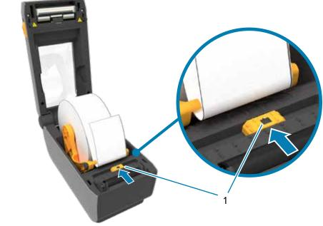
Align the sensor (1) to the center of the roll for regular labels and receipts.
