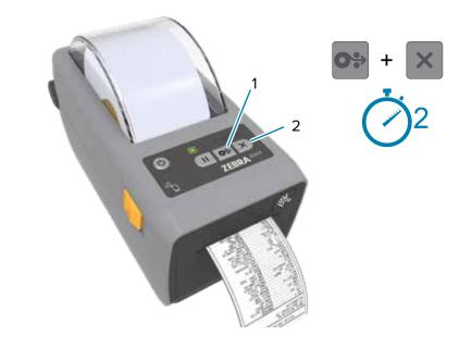
Press and hold the Feed (1) and Cancel (2) buttons for two seconds to print a configuration report.
