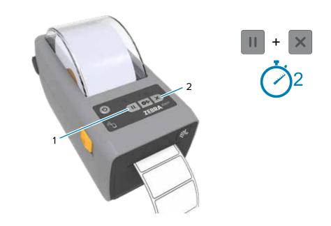
Press and hold the Pause (1) and Cancel (2) buttons for two seconds to line up the labels.
