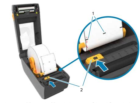
Align the sensor (2) to marks (1) not in the center of the roll for marked labels.
