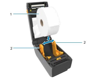
Spread the roll holders (2) open and place the roll (1) into the printer.
