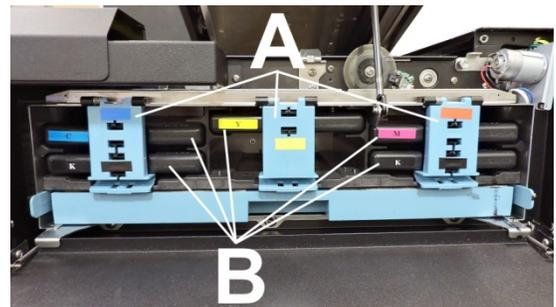
5. **Close Ink Tank Door.** Ink colors fill in as Ink Tanks are installed. If ink colors do not fill in after a few seconds, open Ink Tank Door again and reinstall Ink Tank(s).
