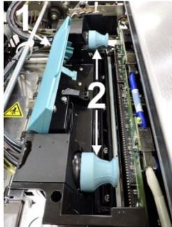
**NOTE: Remove Cap Protectors [2] on Ink Nozzles. Be sure to open Latch fully to retract Ink Nozzles.**
