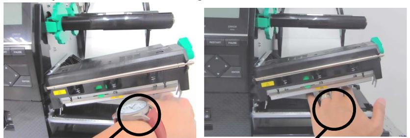
Care must be taken not to allow the metal or glass part of a watch to touch the print head edge.
