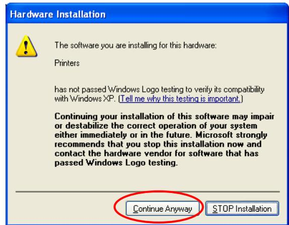
(17) Installation of the printer driver will start.
