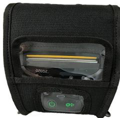
3. Locate the flaps that provide access to the paper path and USB port, and also the opening for the belt clip.
