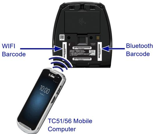
In order to obtain the Bluetooth address or the Wireless LAN address, use a mobile computer to scan the Bluetooth barcode or the WLAN barcode on the bottom of the printer where shown in Figure 23.
