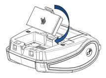
1. Angle the battery pack toward the front of the battery well. The clip on the battery pack should be facing the rear of the printer.
