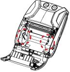
2. Slide the prongs on the back of the spacer into the grooves on each side of the media compartment (circled).
