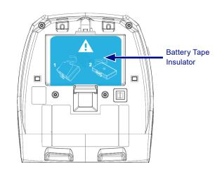
Figure 4 • Removing the Battery Tape Insulator.
