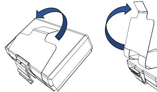
1. Pull up on the tape insulator tab located on the bottom of the battery pack.
