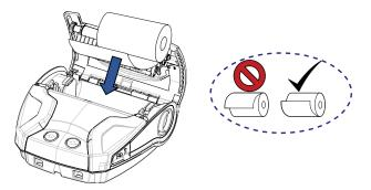
3. Close the media cover making sure to manually feed the end of the media roll outside the printer. The media cover should click into place and the media will then advance on its own.
