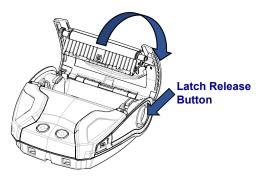
2. Insert the roll of media into the media compartment in the orientation shown.
