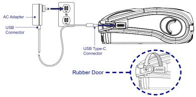
Figure 6 • AC-to-USB Adapter
