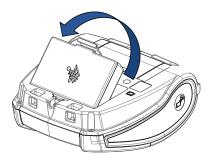
2. Depress the clip on the battery pack and rotate the battery away from the battery well.
