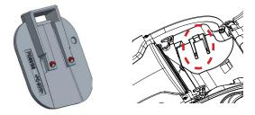
3. Use a flat head tool to insert in the slot at the top of the spacer (circled) to pull up and remove.
