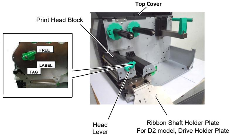
4. Move the Paper Guide R to the rightmost position or shift the guide to the horizontal position.
