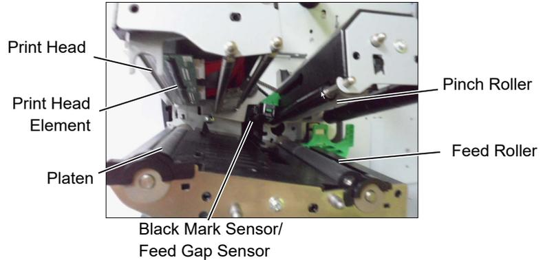
7. Wipe the Platen, Feed Roller, and Pinch Roller with a soft cloth slightly moistened with alcohol. Remove dust or foreign substances from the internal parts of the printer.
