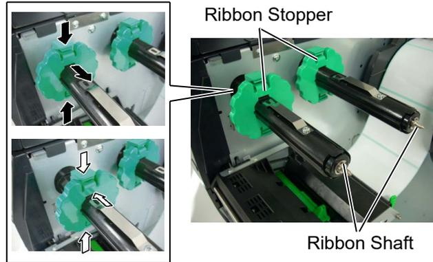
2. Leaving plenty of slack between the ribbon spools, place the ribbon onto the Ribbon Shafts as shown below. There are 2 possible ways to load the ribbon.
