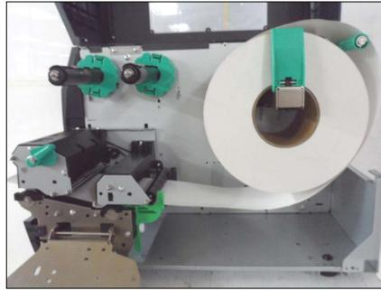
In the case of labels rolled with the print side facing outside.
