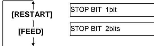
After selecting a stop bit length, press the **[PAUSE]** key.
