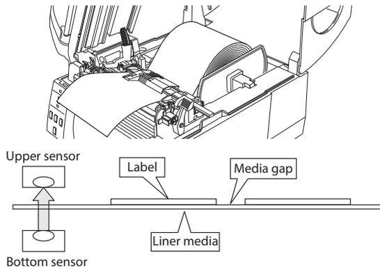
5. If the PAUSE key is pressed and released while the MODE/ REPEAT key is pressed, the PRINT LED goes off, after the CONDITION LED switches from lit to flashing, media feeding starts, and the sensor is automatically adjusted.
