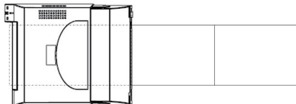
Place the fanfold media so that it is parallel with the printer.
