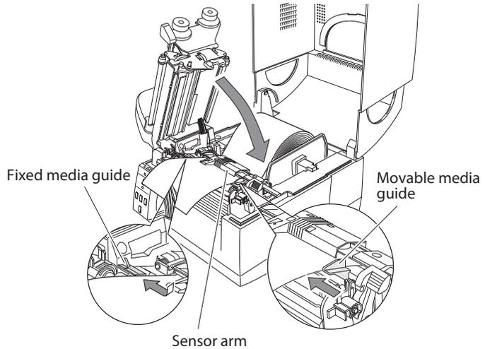
9. Push the head close knob to lower and lock the head unit. Be sure to always push the head close knob to lock the head unit. Align it with the width of the media that has been set, then set the media width and media thickness adjustment dials. See "Chapter 3 Printer Adjustments".
