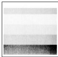
The first sample, left, shows an incorrectly set “media thickness adjustment”. For standard label media, it is recommended you set the blue dial to the “0” position.
