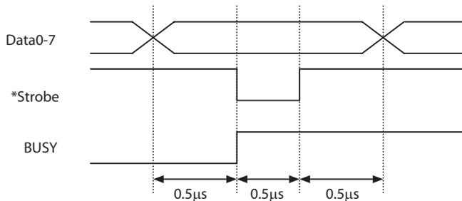
**Note:** Busy rises when \*Strobe signal starts, and data is latched with \*Strobe signal starts.
