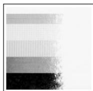
The second sample, left, shows an incorrectly set “media width adjustment”. For 4-inch or 100mm wide media, the adjuster should be set to the “9” position on the blue dial.
