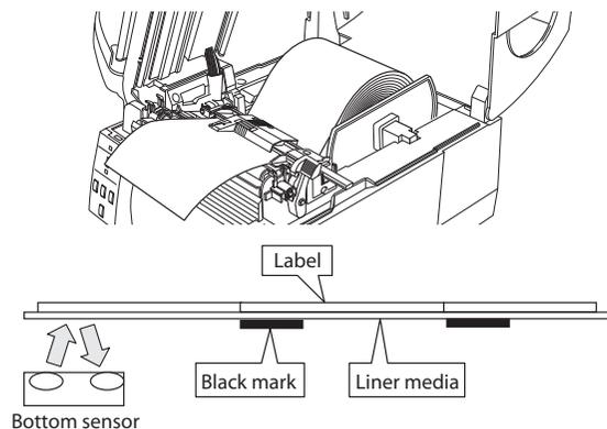
4. If the PAUSE key is pressed and released while the MODE/ REPEAT key is pressed, the PRINT LED goes off, after the CONDITION LED switches from lit to flashing, media feeding starts, and the sensor is automatically adjusted.
