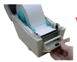
Refer to section 3.2 to load the media. Open the top cover and peeloff panel after calibrating the sensor.
