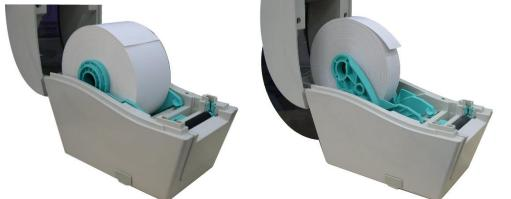
**4.** Place the roll between the holders and close them onto the core.
