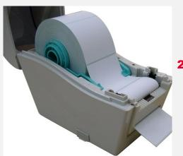
2. Push the peel-off panel back to the printer.
