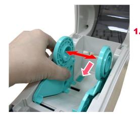
Open the printer's top cover and separate the media holders to fit the media width. Press down the media holder lock switch to fix the media holder.
