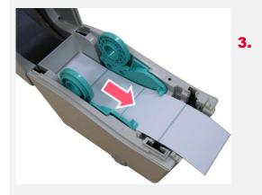
Place the paper, printing side face up, through the media guides, media sensor and place the label leading edge onto the platen roller.
