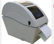
Close the top cover gently and make sure the cover latches securely, calibrating the printer by hardware or software. (Refer to Chp.4&5)
