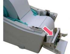
**3.** Lead the media through the backing paper opening beneath the peel-off roller.
