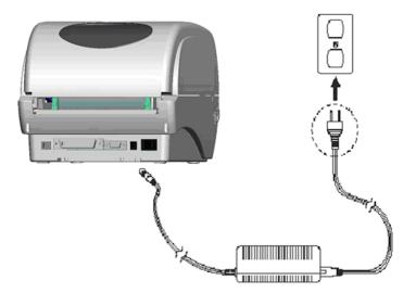
Note: Please switch OFF the printer before plugging in the power cord to printer power jack.
