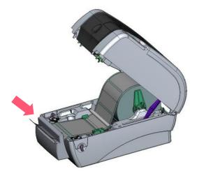
**5.** Close the top cover by lifting up the top cover support and close the top cover slowly.
