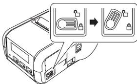
2. Insert the battery into the battery compartment until the battery latch locks into place. Make sure that the terminal end of the battery is facing inwards and oriented correctly as shown. Do NOT use excessive force to install the battery.
