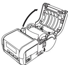
2. While pushing the roll release lever, tilt the roll guide slightly, and then remove the roll. The roll can be removed without changing the position of the roll guide. Do not forcefully tilt the roll guide too far. Otherwise, the roll guide could break.
